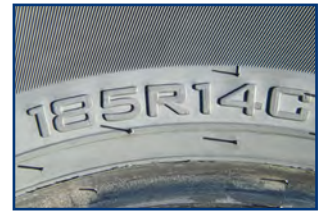
Markings on a 185R14C commercial tyre.
