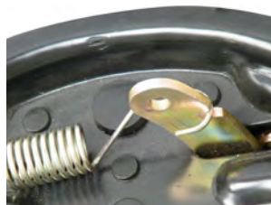
◀ Mechanical park brake lever shown.
