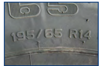
Markings on a 195/65R14 passenger car tyre.
