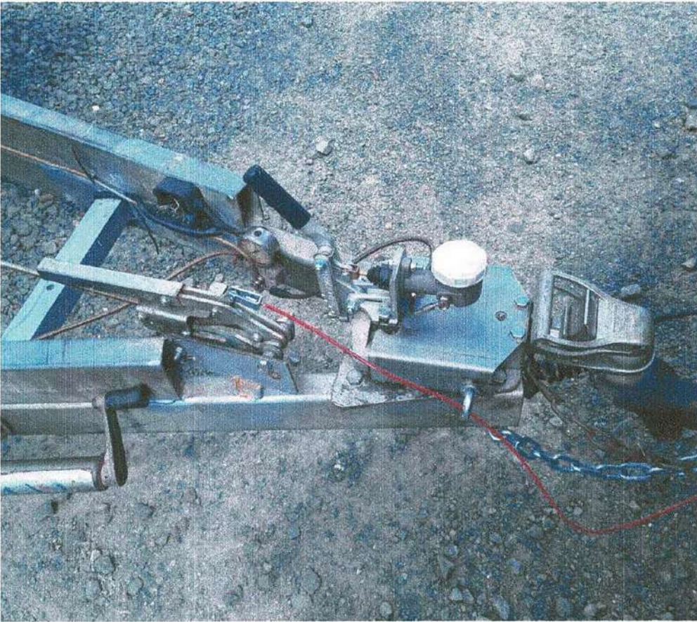
Figure 2 – Hygo 3 breakaway brake activation. Note breakaway cable guide
